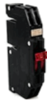
Zinsco R3820 20A 2-Pole 120/240V Circuit Breaker (used) Description : 120VAC : 10k, Voltage : 120/240VAC, Terminal Connection : Lug, Phase Connection : A, Min. Wire Size (AWG) : 14, AIR Rating : 10k, Type : Panelboard Mount, Circuit Breaker
